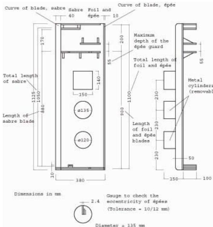
Figure 16. Gauge for checking weapons
