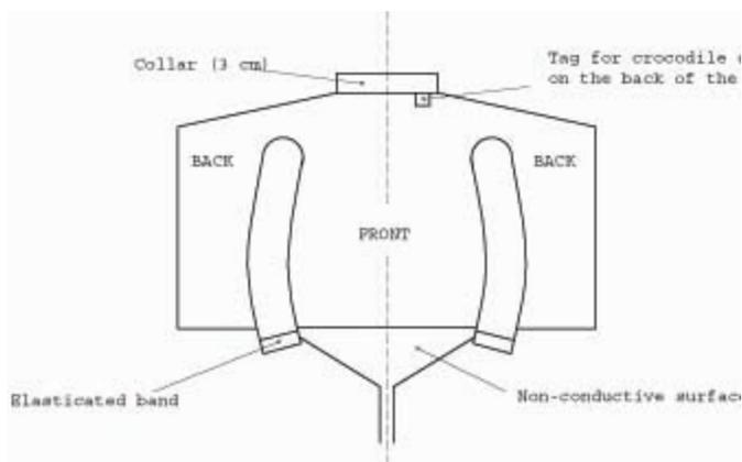
Figure 15. Electric saber conductive jacket
