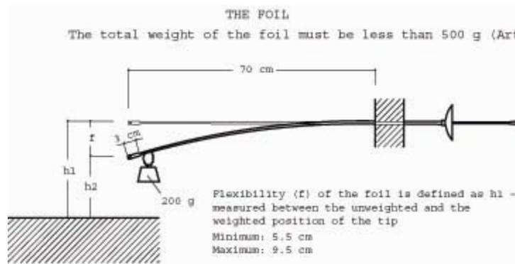
Figure 8. Foil dimensions and flexibility
