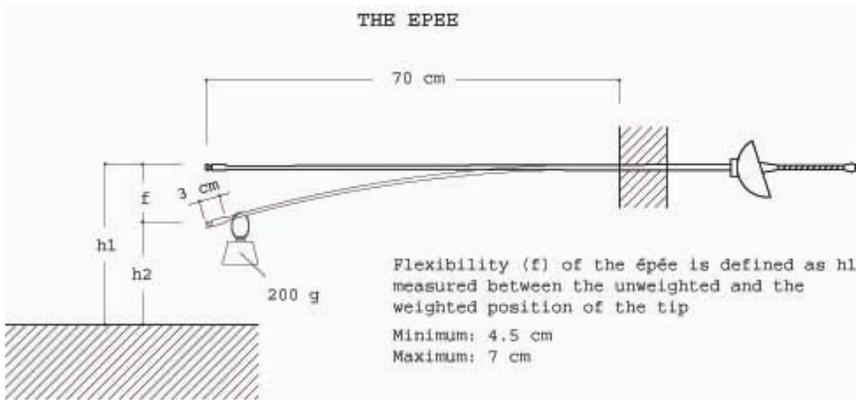
Figure 9. Epee dimensions and flexibility
