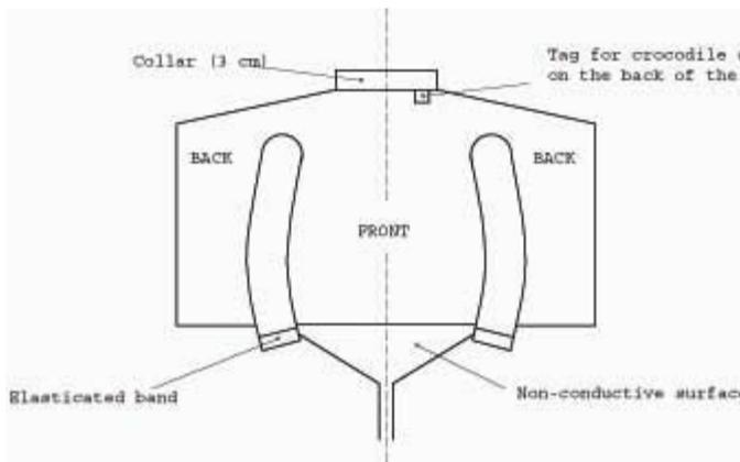
Figure 15. Electric saber conductive jacket
