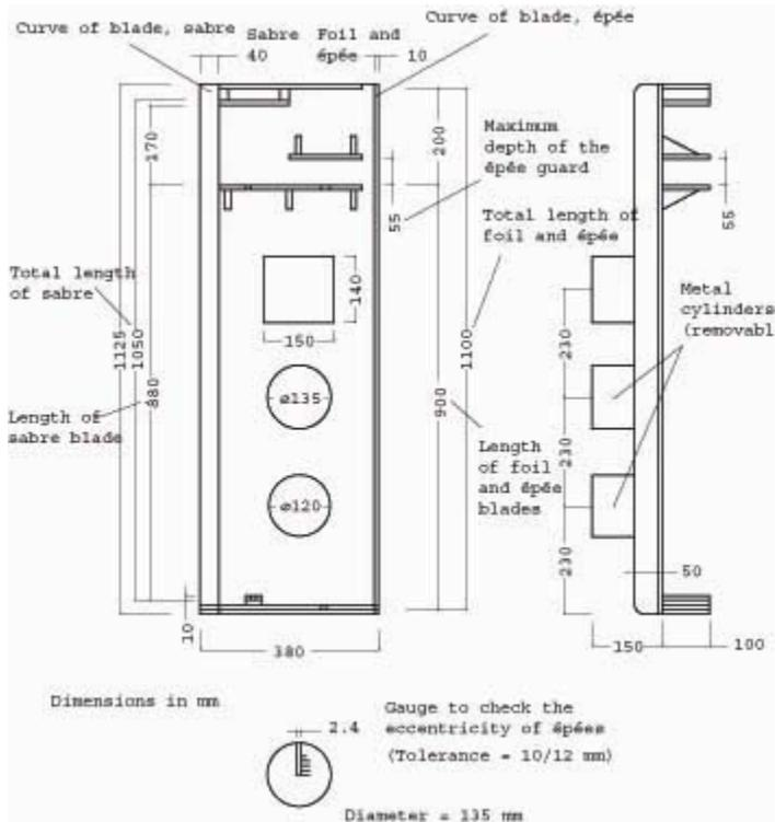
Figure 16. Gauge for checking weapons
