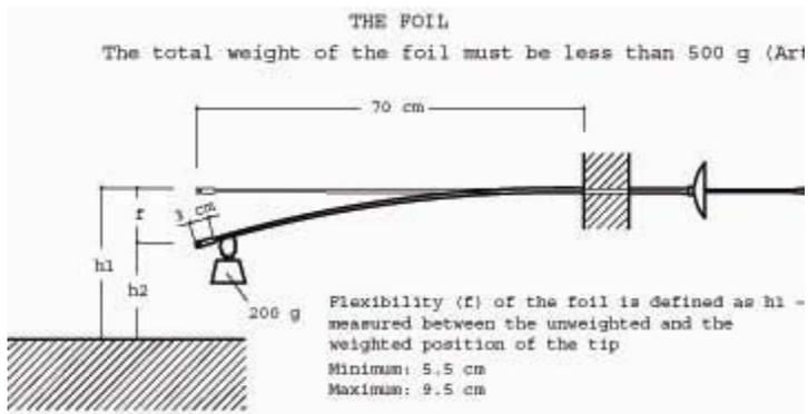
Figure 8. Foil dimensions and flexibility
