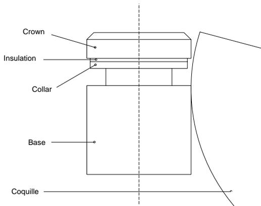
**Figure 11. Épée: details of tip of point**
