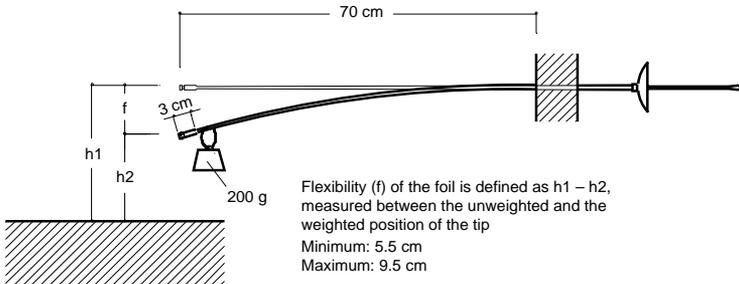
**Figure 8. Foil dimensions and flexibility**
