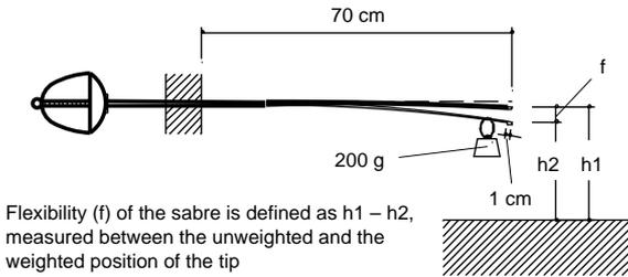
Flexibility (f) of the sabre is defined as  $h1 - h2$ , measured between the unweighted and the weighted position of the tip
