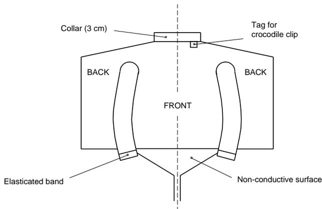
**Figure 15. Electric sabre: conductive jacket**
